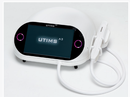
LCD touch screen 10 inches 6 Transducers HIFU for face. 6 Transducers HIFU for body. Compatible with CENTERLESS System.
